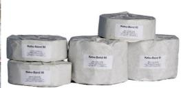
Kebu Tape 90 consists of a synthetic fibre fabric liner (100 g/m²) impregnated and coated with a neutral compound based on petrolatum and inert siliceous fillers. During application, a spiral wrapping with overlapping must be performed. After wrapping, the surface and especially the edges must be smoothed. This can be done by hand. Every overlap must be tightly sealed. If required, an additional outer layer of Kebulen-PE foil 0.25 or 0.40 can be applied as mechanical protection.
